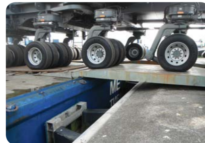
Self propelled crane rolling onboard mv MERI by using ship's portable ramp elements
