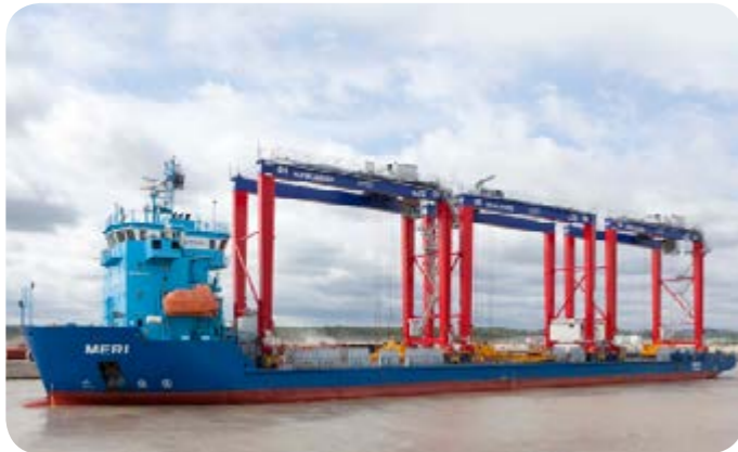
Rubber tyred container gantry cranes North Europe Sea transport, engineering, sea fastening
