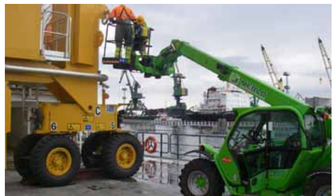
Vessels are equipped with telescopic forklift for handling of equipment's onboard and giving access to higher location.
