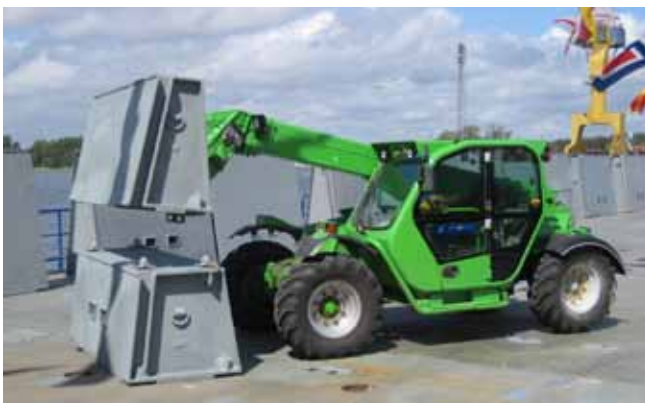
Vessels are equipped with telescopic forklift for handling of equipment's onboard and giving access to higher location.
