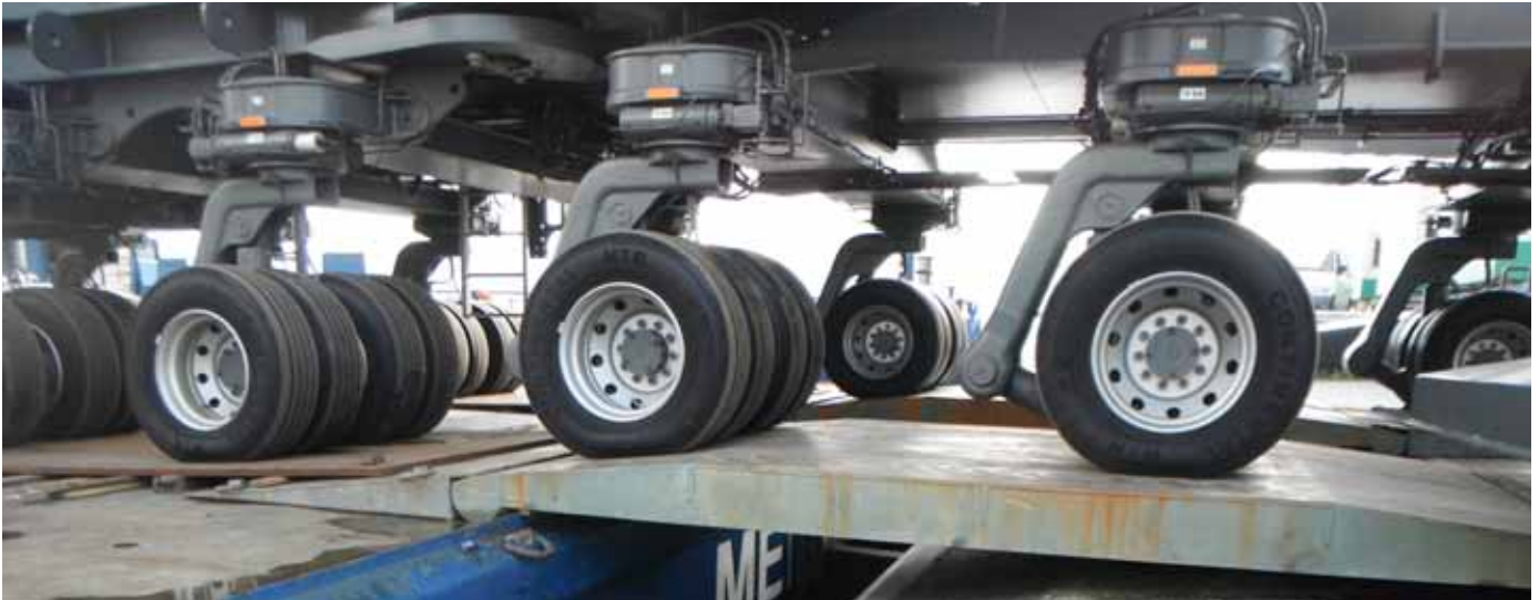
Self propelled crane rolling onboard mv MERI by using ships portable ramp elements
