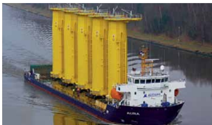
Windmill transition pieces Germany / UK Fabrication of transportation frames and sea transport
